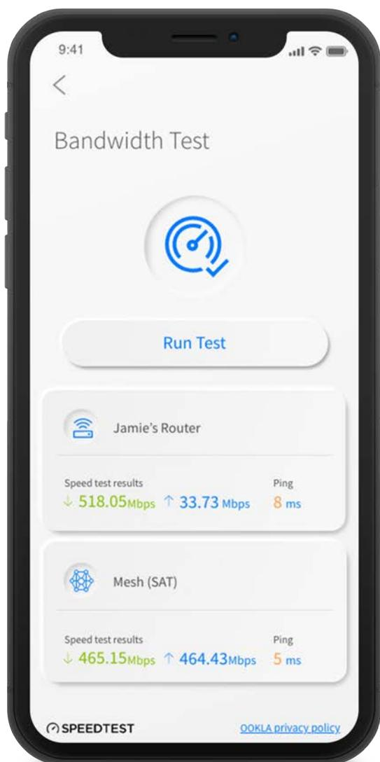
The easiest way to run a bandwidth test is by tapping into “My Network” from the main dashboard and then tapping into your Wi-Fi router. Tap “Bandwidth Test” in the Settings section. Then hit the “Run Test” button.
